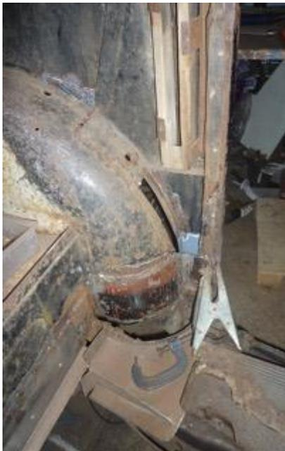
Serious repairs to rear wheel arch
