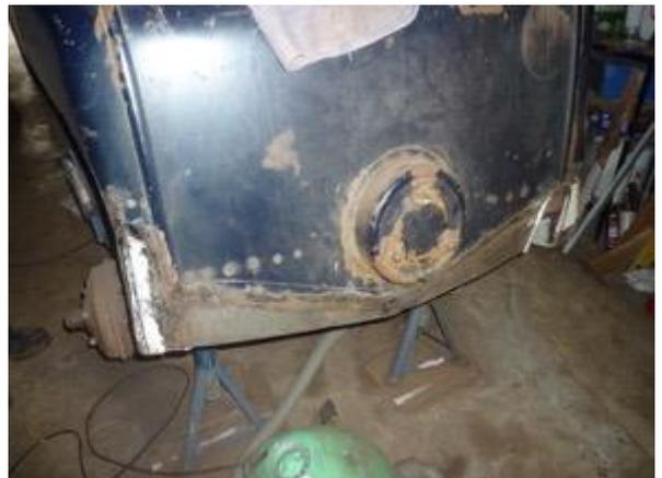
**New bottom edge welded in position**
