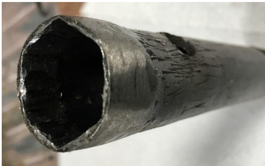
Box spanner for cutting the split pin in the front stub axle
