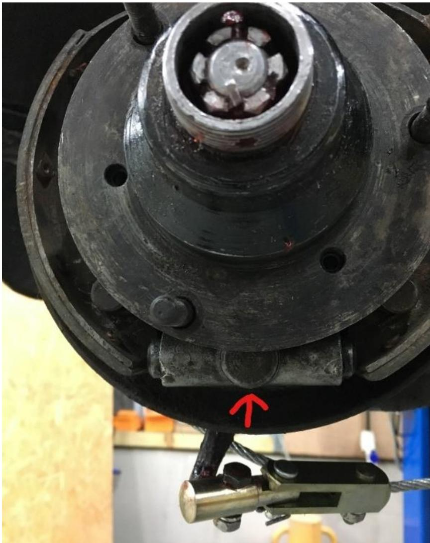
*Cam (red arrow) cannot be removed without removing hub first. Photo after rebuild, showing front nearside hub, with lever now resting in forward facing position.*
