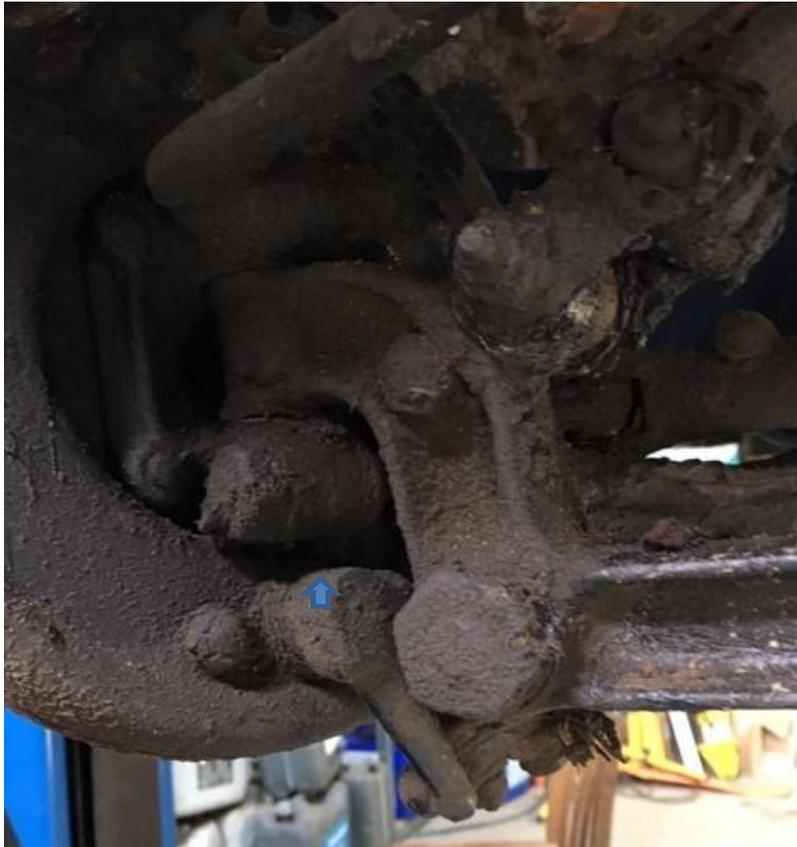
*The front brake lever (offside) prior to rebuild, in resting mode, pointing towards the brake cable. Compare to next picture following rebuild.*
