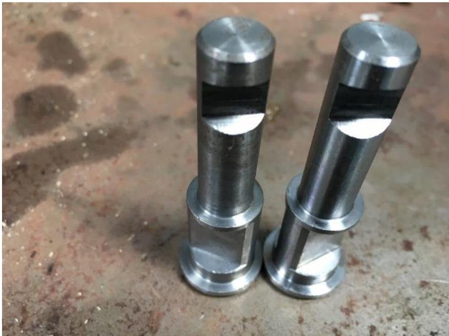
*Note different alignment of the cams for each side. The upper indentations are for the cotter pin which attaches them to the brake lever, and the lower ones are the cams that push the pistons that in turn push on the brake shoes.*
