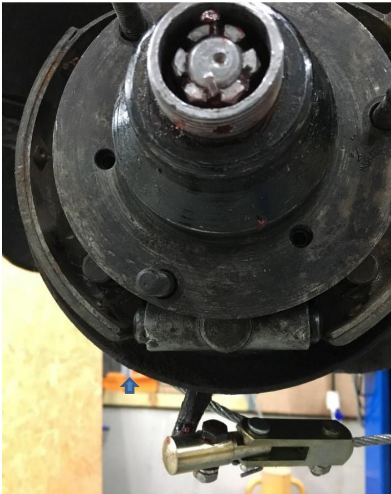
*Following rebuild, brake cable (nearside) now pointing forwards (away from brake cable)*
