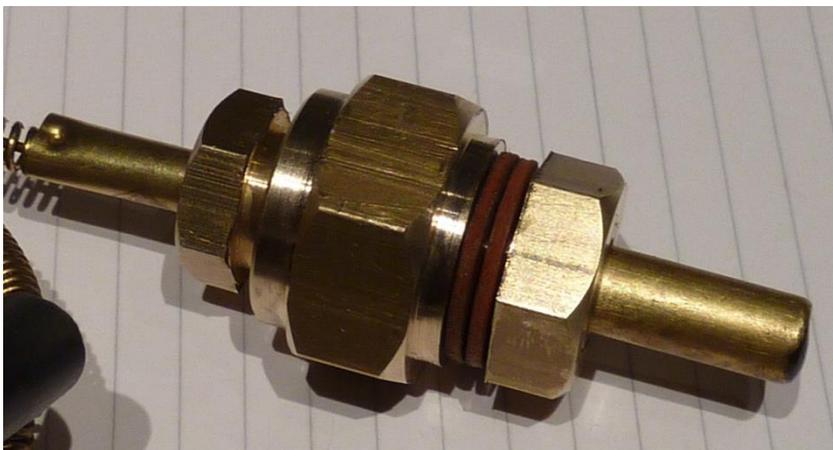
So, then, it was simple task of turning-up an adapter bush (from 1" AF brass hexagon) to accept the sender and include a male threaded spigot to pass through a 1/2" hole in the tank wall. The bush was secured with a fibre washer either side of the tank
