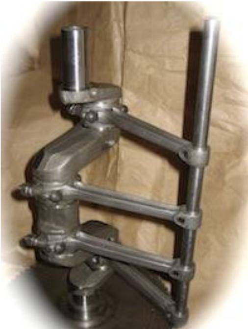
When assembling an Austin Seven engine, it is very easy to check whether your con' rods are sufficiently straight. I understand alignment within two thou' over 4 inches length is deemed an acceptable tolerance.
