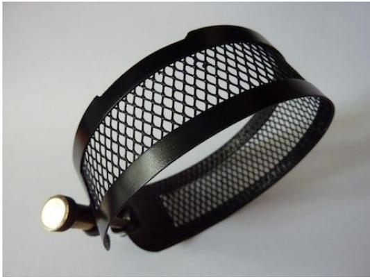
Another item of possible interest is this recently spotted dynamo brush cover. Clearly not for the purist but it could be useful anyone pushing a six-volt dynamo really hard by winding the third brush a long way anti-clockwise (looking at the distributor end of the dynamo) to maintain charge whilst using uprated headlight bulbs together with an electric wiper motor.
